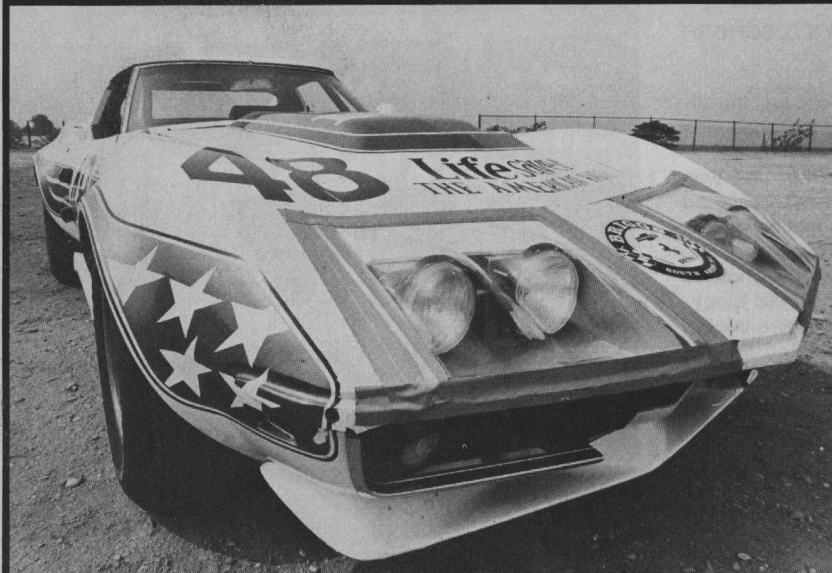
Headlight fairings aren't legal in all states but they sure look neat. Interior sports one race seat and one street seat and full safety equipment. Hurst shifter is surrounded by switches and warning lights. All lines are of braided steel aircraft material and the suspension is an exact dupe of one used in race cars. Even the chassis is a jig-built affair. Wheels are super-expensive, super-light Minilite mags.
